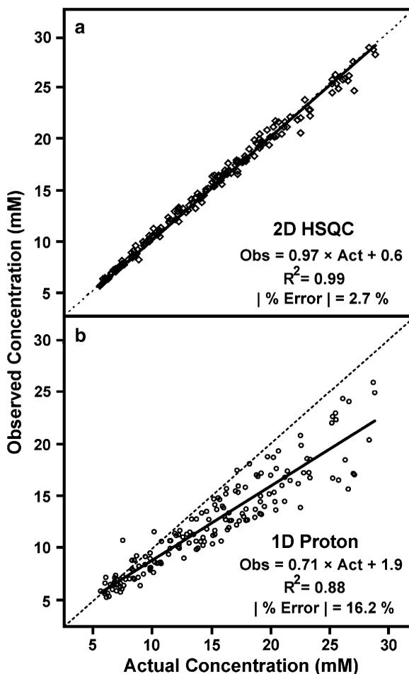
Fig. 7. (a) Concentration estimates ( $N = 168$ ) based on two-dimensional  $^1\text{H}$ - $^{13}\text{C}$  HSQC and (b) one-dimensional  $^1\text{H}$  NMR data. Estimates are plotted as a function of the known concentration of metabolites in synthetic mixtures. Dotted lines indicate the ideal regression (slope 1), and the solid lines indicate the best-fit regression.
