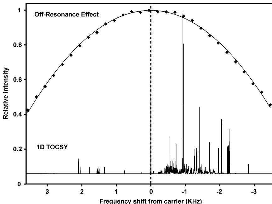
Fig. 6. Off-resonance effects are one of the many factors that can influence peak intensities observed in NMR experiments. In this example, the intensities in  $^1\text{H}$ - $^1\text{H}$  TOCSY were measured as a function of  $^1\text{H}$  frequency offset. The peak intensity is highest when the peak is closest to the transmitter frequency and lowers as the transmitter is tuned to higher or lower frequencies.
