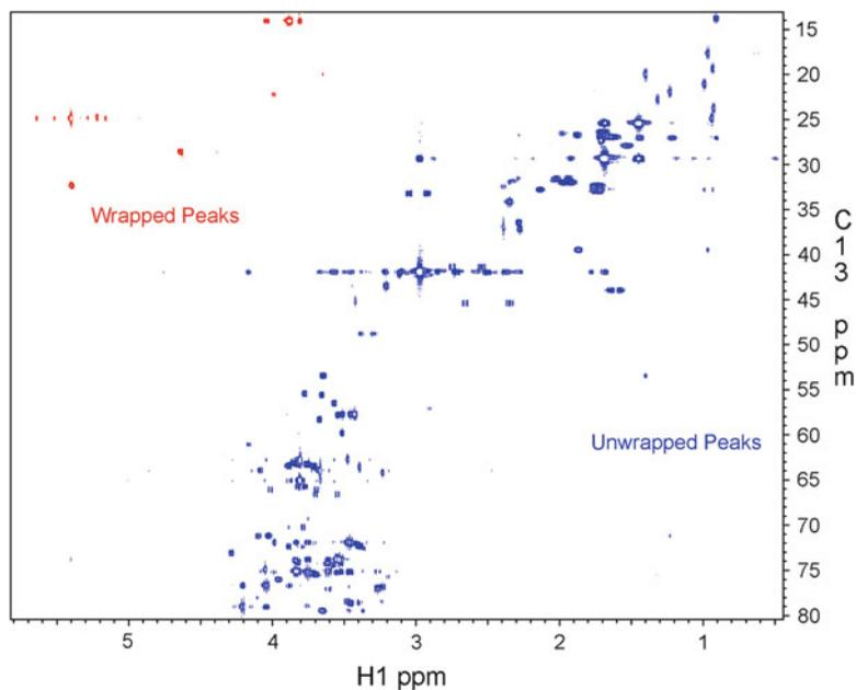
Fig. 8. Quantitative  $^1\text{H}$ - $^{13}\text{C}$  HSQC NMR spectrum of a synthetic mixture of 26 metabolites. The spectral width in the indirect dimension was reduced to allow for shorter acquisition times. *Blue peaks* are in their correct locations, whereas *red peaks* have been wrapped into the top of the spectrum from their normal downfield positions.
