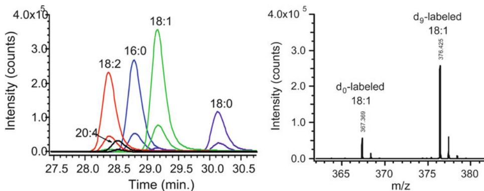
Fig. 3. Representative extracted ion chromatograms and a mass spectrum for cholamine-labeled fatty acids (1). Light and heavy labeled fatty acids coelute from reverse phase LC (*left*) and are easily distinguished by MS by their characteristic 9 Da shift (*right*). Amines labeled as shown in Fig. 2 yield analogous results.
