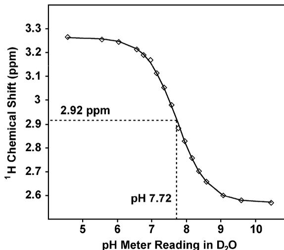
Fig. 1. The  $^1\text{H}$  chemical shifts of several HEPES peaks are pH sensitive and can be used as an internal pH reference. The titration curve was generated from a HEPES buffered saline solution (290 mOsm) in  $\text{D}_2\text{O}$ . The *dotted lines* indicate the observed  $\text{p}K_a$  of HEPES as an uncorrected meter reading in  $\text{D}_2\text{O}$ .
